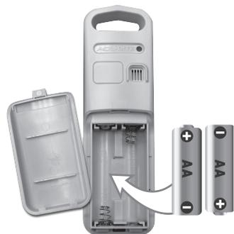
1. Slide off the battery compartment cover.
