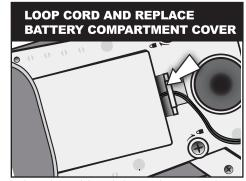
Loop the cord through the slot, then replace the battery compartment cover
