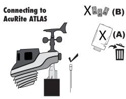
The included IRIS battery compartment adaptor (A) and wire routing clips (B) will **NOT** be utilized for installation with the AcuRite Atlas.
