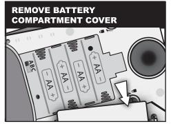
Remove battery compartment cover from the bottom of the AcuRite Optimus outdoor sensor. Remove batteries if currently installed.
