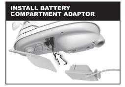
Install the wired battery compartment adaptor into the AcuRite Iris Sensor.
