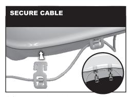
To further secure the wired battery compartment adaptor to the AcuRite Iris Sensor and prevent the wire from interfering with the wind vane, insert the (3) in-line clips into the 5-in-1 Sensor as shown.
