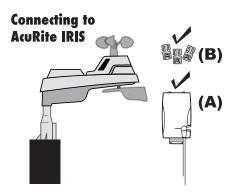
The included IRIS battery compartment adaptor (A) and wire routing clips (B) will be utilized for installation with the AcuRite Iris (5-in-1).
