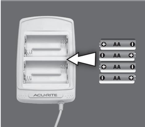
5. Insert 4 x AA alkaline or lithium\* batteries into the battery compartment. Heavy duty or rechargeable batteries are not recommended.
