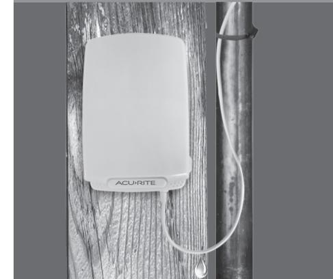
7b. Use the included zip ties and hardware to secure excess cable near the battery pack, leaving enough slack for a "drip-loop," preventing rain water from trailing into the battery pack. Installation is complete.
