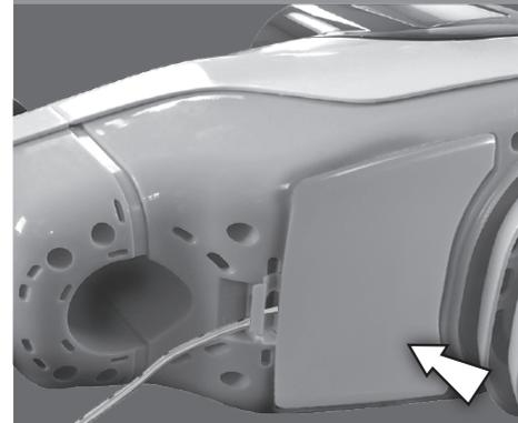
3. Loop the cord through the slot, then replace the battery compartment cover.
