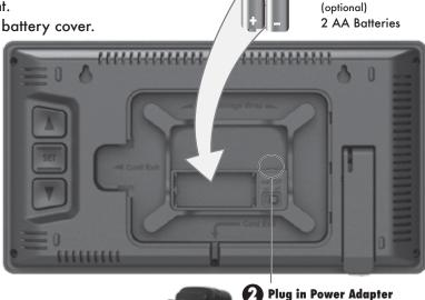
IMPORTANT: Batteries are a backup power source to preserve records in the event of a power outage. Power adapter is required as the power source of this product.
