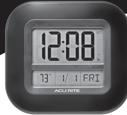
**NOTE:** A clear protective film is applied to the LCD at the factory that must be removed prior to using this product. Locate the clear tab and simply peel to remove.
