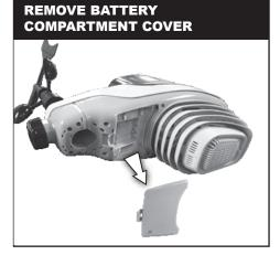
Remove battery compartment cover from the bottom of the AcuRite<sup>®</sup> Atlas<sup>™</sup> outdoor sensor. Remove batteries if currently installed.
