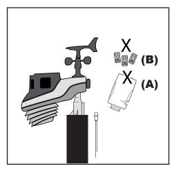
4. The included battery compartment adaptor (A) and wire routing clips (B) will NOT be utilized for installation with the AcuRite Atlas. If you have an AcuRite ATLAS sensor, you may unplug the battery compartment adaptor and discard it.
