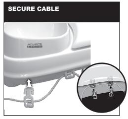
7. To further secure the wired battery compartment adaptor to the AcuRite Iris Sensor, insert the three (3) in-line clips into the 5-in-1 Sensor as shown. The cord must be taut along the base of the sensor to prevent it from interfering with the sensor's wind vane.
