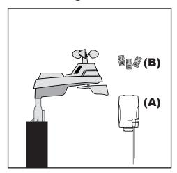
The included battery compartment adaptor (A) and wire routing clips (B) will be utilized for installation with the AcuRite Iris (5-in-1).
