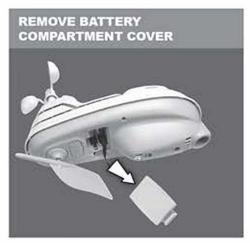
Remove battery compartment cover from thee bottom of the 5-in-1 Sensor (keep or discard).e Remove batteries if currently installed.e
