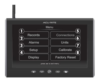
Navigate to the main menu at any time by pressing the "\operation" button. From the main menu, you can view records, set alarms, setup an additional sensor and more.
