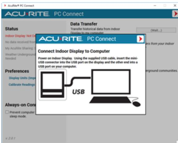
3. From the Status section, verify the **Indoor Display** status changed to **Detected**.
